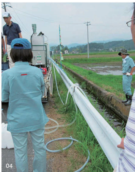
[01] Sampling at Nagadoro agricultural pond in Iitate Village [02] A high-speed continuous centrifugal pump for sampling suspended matters [03] Radiocaesium extraction from bound-to-organic fractions by decomposition [04] Sampling of suspended matters in agricultural water at Ota in Minamisoma City [05] Laboratory experiment to study the transfer of radiocaesium from soil/water to rice [06] Sampling at a reservoir in Nagadoro, Iitate Village [07] Sampling of agricultural water using a submersible pump [08] An irrigation canal in Ota area, Minamisoma City
