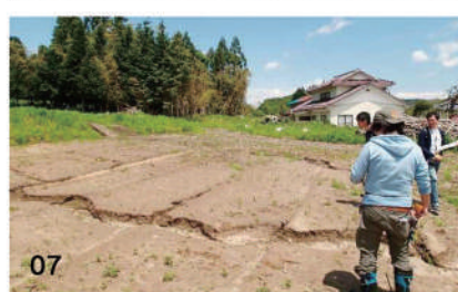
[01] Setting up an artificial grass mat on Niida River floodplain [02] Water sampling from an irrigation pond [03] Dose rate survey of the waterfront park [04] Study of the Niida River floodplain [05] Runoff plot [06] Surface runoff and soil erosion during heavy rain [07] Decontamination site eroded by rainfall [08] Sampling of suspended sediments in the river
